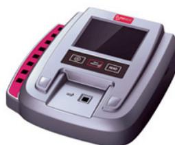
Halo BIOMaster allows measurement of nucleic acid concentrations and purity (using ratio function) including protein concentrations. As a high quality spectrophotometer, the Biomaster features touch screen operation packaged as a lightweight system with a compact footprint for life science and education related applications.
